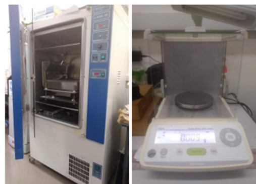
a) Temperature-humidity control cabinet and electronic scale
