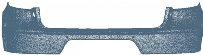
Figure 2. Point cloud data of the rear bumper component used as the experimental case study
