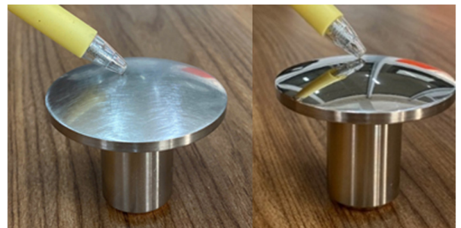
Figure 8. Spherical workpiece surface before and after polishing
