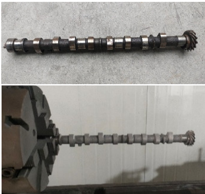
Figure 8. Details of the camshaft before and after HVOF injection
