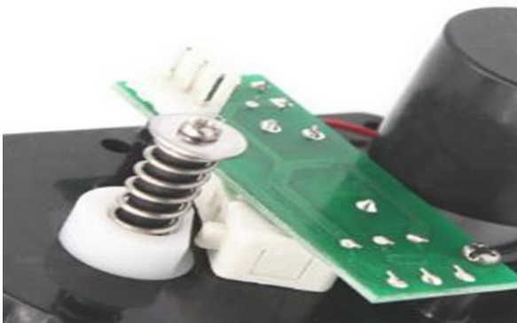
Figure 5. Mechanical arrangement of the cam disk and the snap-action limit switch
