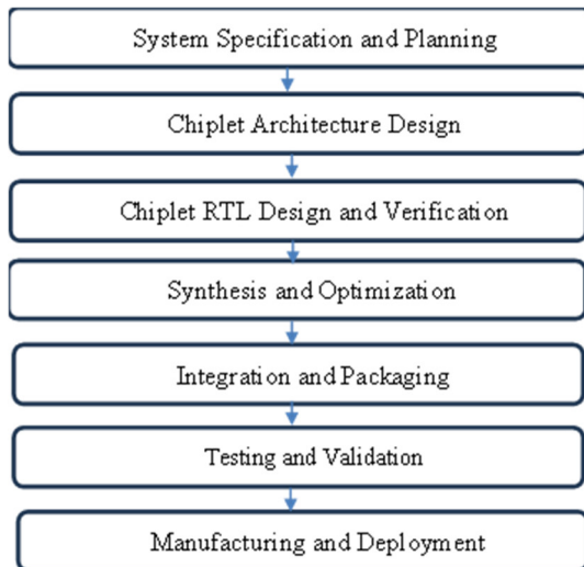
Figure 2. Chip Design Flow with Chiplet Technology
