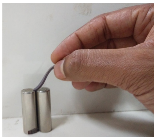
Fig. 5. The Ferrogel cantilever deflected towards a permanent magnet
