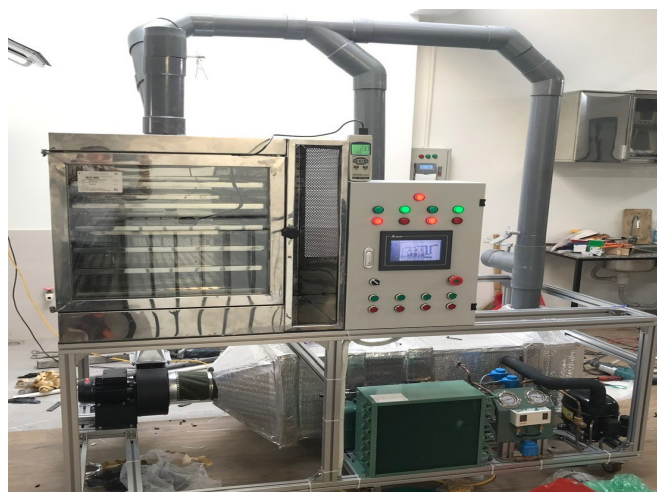
Fig. 1. Schematic diagram of the combined heat pump - hot water solar dryer used in this study
