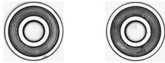
c) Type 3: Scratch/Edge defect
