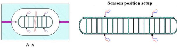
Fig. 3. Attached thermocouple in the test section
