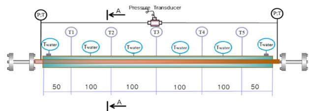
Fig. 2. Details of test section
