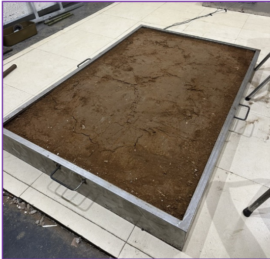
Fig. 8. The platform for the shot (soil tray) is compacted
