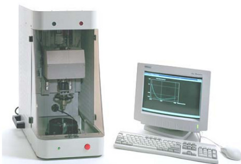
Fig. 4. UTM-2 Friction Measurement Device
