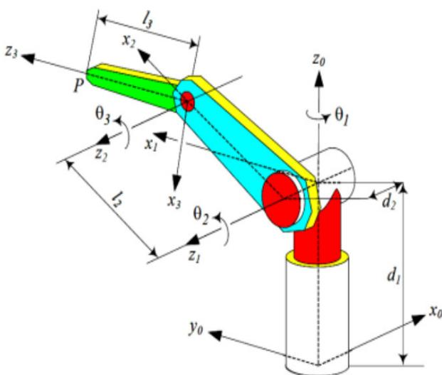
Fig. 2. The structure of a robot with 4-links and 3-joints [1,8]
