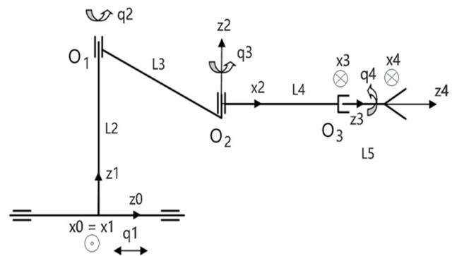
Fig. 3. The kinematic diagram of the picking arm robot
