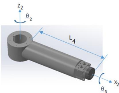
Fig. 7. The L4 link arm assembly
