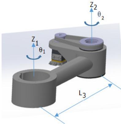
Fig. 9. The  $L_3$  link elbow assembly
