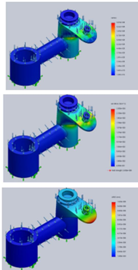
Fig. 10. The strength analysis results of three design options of the  $L_3$  link
