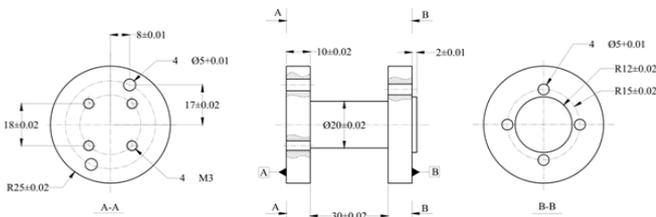
Fig. 6. The L5 link arm assembly
