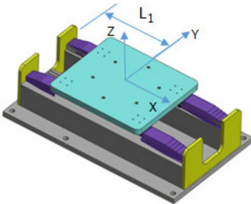
Fig. 13. The structure of the robot base assembly (L<sub>1</sub> link)
