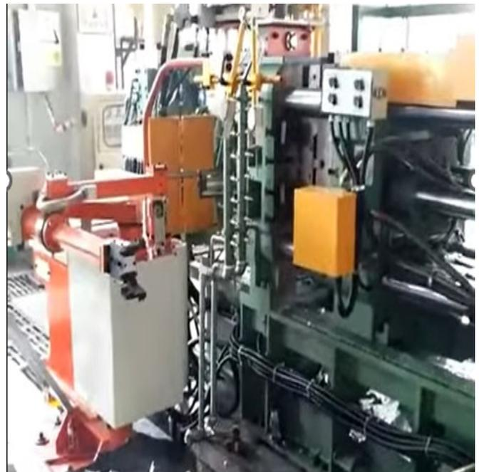
Fig. 1. A picking robot working on a pressure casting machine [9]
