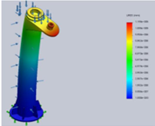
Fig. 12. The strength analysis results of three design options of the L<sub>2</sub> link
