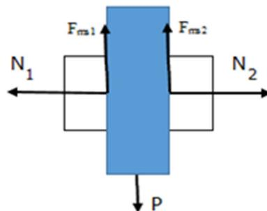
Fig. 5. The analysis model of the force components acting on the picking arm and product
