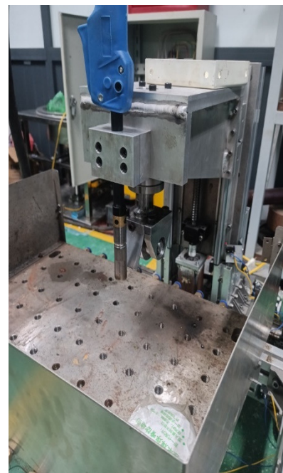
Fig. 3. The metal 3D printer integrated rolling mechanism
