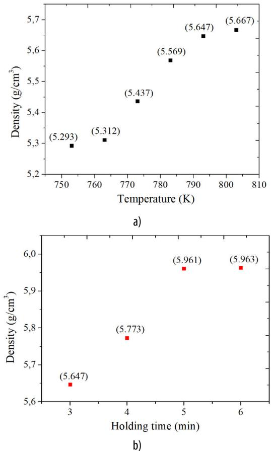
Fig. 2. Effect of temperature (a) and holding time (b) on dense level of TiZr-based BMGF
