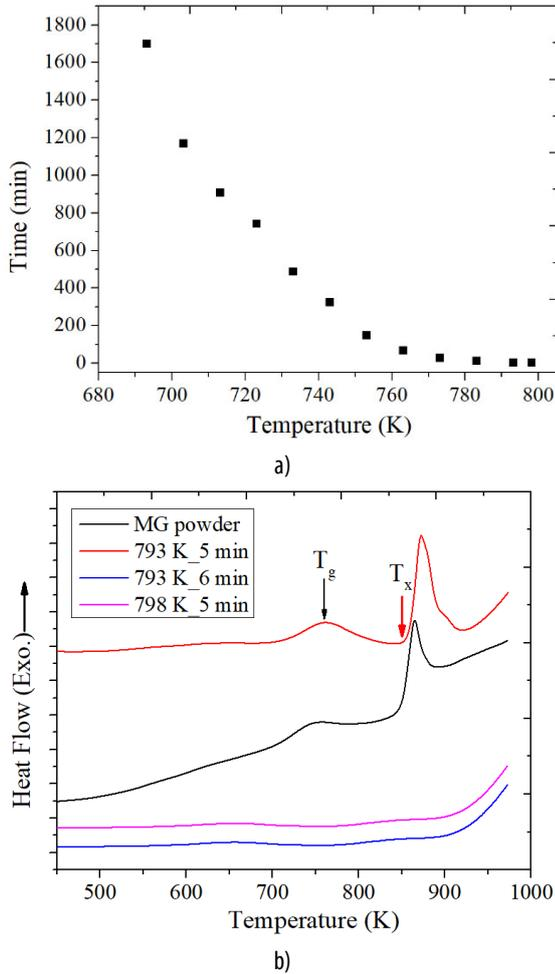
Fig. 1. (a) Incubation time of MG powder under different isothermal annealing experiments; (b) DSC traces of MG powder after the isothermal annealing at the various temperatures and holding times
