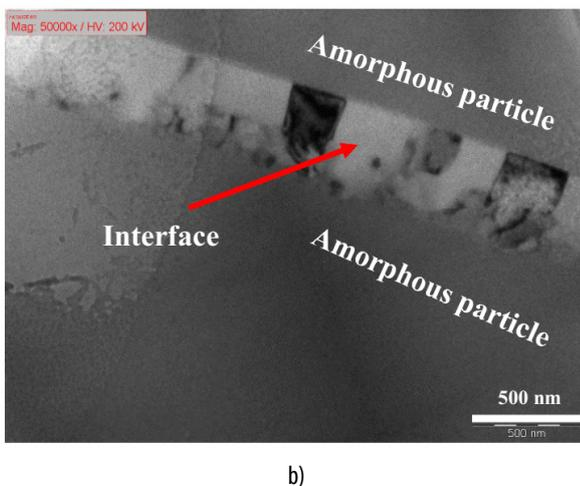
Fig. 3. (a) XRD patterns of MG powder and TiZr-based BMGFs produced at the different temperatures and holding times; (b) Bright-field TEM image of interface between the amorphous alloy particles
