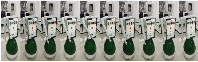
Fig. 3. Robot's right arm movements to perform the handshake task with the interactor
