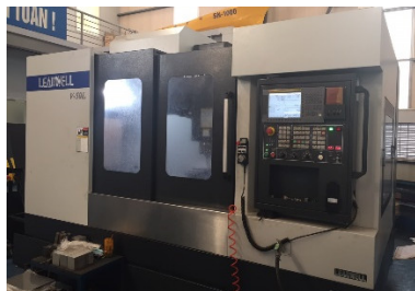
Fig. 5. LEADWELL V-50L machining Center
