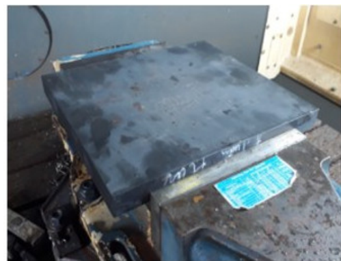
Fig. 1. SKD11 alloy steel workpiece after heat treatment
