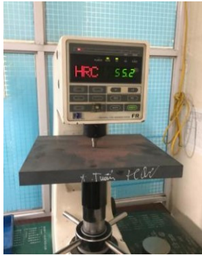
Fig. 3. Hardness Tester FR-1E Machine
