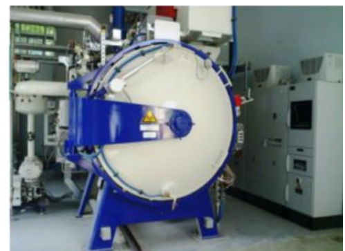
Fig. 2. Turbo-IPSEN heat treatment equipment
