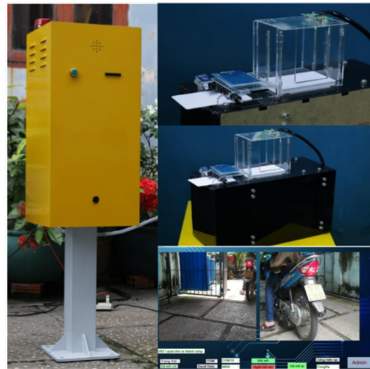
Fig. 4. Automatic Card Issuance Booth and Box; Management Interface
