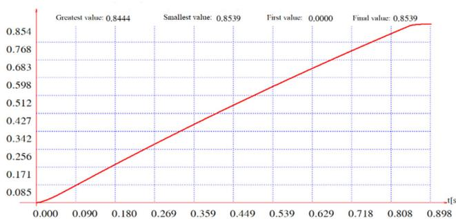
Fig. 7. Total amount of gas ejected through the nozzle over time
