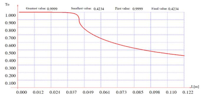
Fig. 10. Graph of the temperature of the combustion gas along the nozzle length
