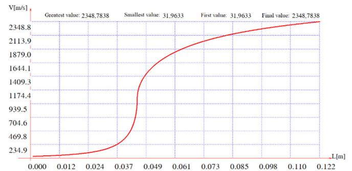
Fig. 8. Graph of the velocity of the combustion gas along the nozzle length
