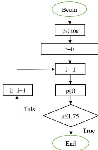
Fig. 3. Algorithm diagram for determining the working parameters of the combustion chamber in the free gas injection phase
