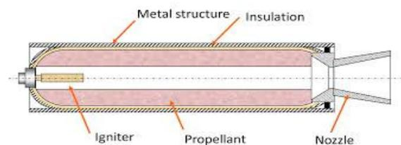
Fig. 1. General structure of rocket engine
