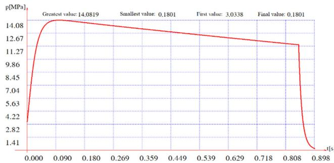
Fig. 5. Working pressure in the engine combustion chamber over time
