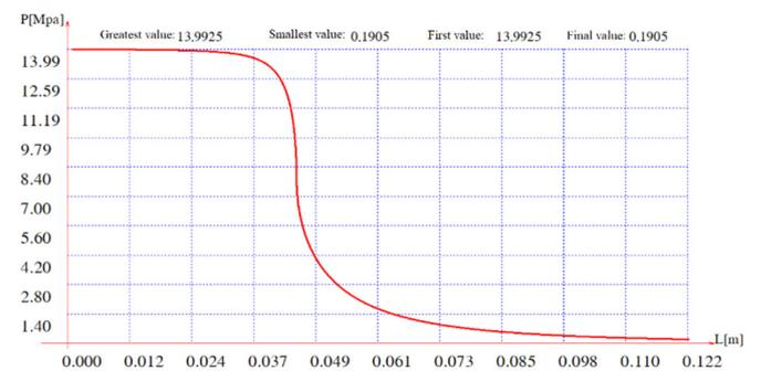
Fig. 9. Graph of the pressure of the combustion gas along the nozzle length
