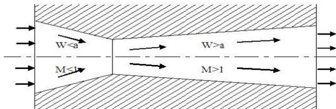
Fig. 4. Laval nozzle diagram
