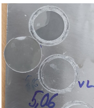
a) After pull-off test
