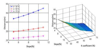
Figure 4. Investigation of braking distance with road gradients ranging from 5% to 11% and pedal brake travel ratio k varying from 30 to 70% (supplementary brake torque  $M_b = 80$ Nm; adhesion coefficient  $\phi = 0.7$ ,  $v_1 = 60$ km/h,  $v_2 = 20$ km/h)
