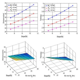
Figure 2. Investigation of braking distance and braking time with road gradients ranging from 5% to 11%, supplementary brake torque M<sub>b</sub> varying from 20 to 80Nm (adhesion coefficient  $\varphi = 0.7$ ,  $v_1 = 60$ km/h,  $v_2 = 20$ km/h, pedal brake travel ratio k = 50%)
