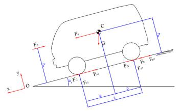
Figure 1. Forces and moments acting on van truck when descending a slope and braking
