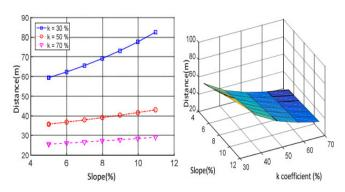
Figure 3. Investigation of braking distance with road gradients ranging from 5% to 11% and pedal brake travel ratio k varying from 30 to 70% (supplementary brake torque  $M_b = 20Nm$ ; adhesion coefficient  $\phi = 0.7$ ,  $v_1 = 60km/h$ ,  $v_2 = 20km/h$ ).
