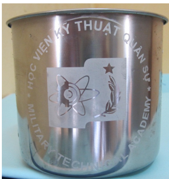
Figure 5. Logo marking on thin-walled product
