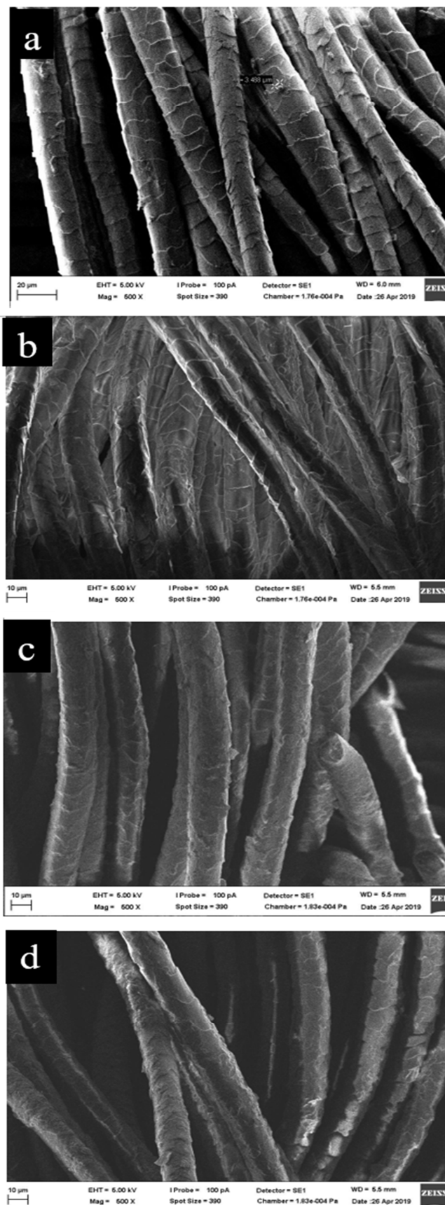
Figure 3. Sample SEM images: a) unwashed, b) after 1 wash, c-d) after 5 washes
