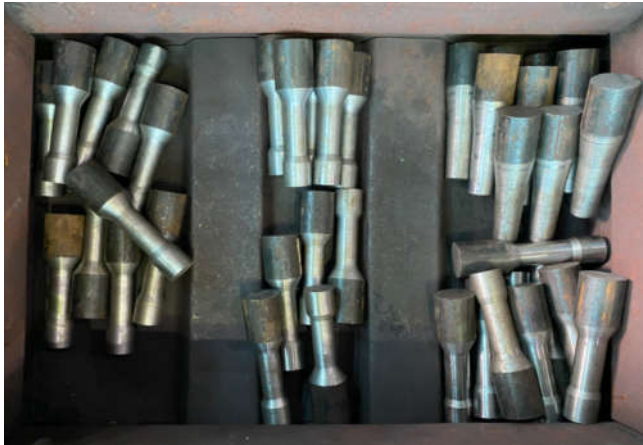
Fig. 4. Actual workpieces for forging experimental
