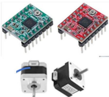
Figure 13. A4988 stepper driver and engines
