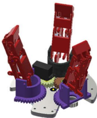
Figure 6. 3D model of the fingers
