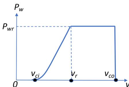
Fig. 2. The power curve of a wind turbine
