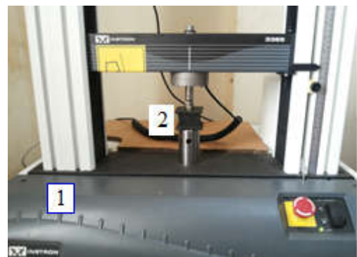
Figure 2. Stiffness testing of the mount
